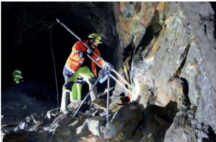
Image 1: Geophysical borehole logging at Koralpe lithium exploration mine, Wolfsberg, Styria, Austria
