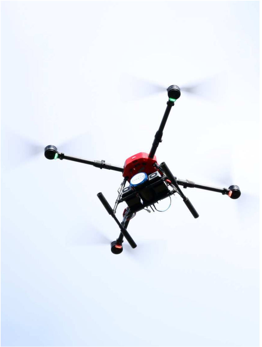
Image 2: Drone-borne mapping system while surveying.
