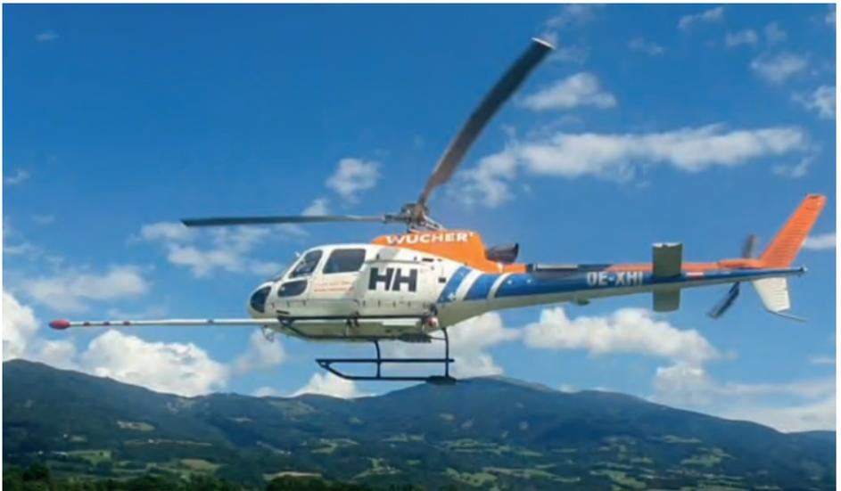
Image 1: Magnetic and radiometric nose boom system on survey in the Austrian alps '23.
