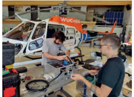
Image 2: terratec data acquisition system and spectrometer rack mounted in the rear of an Airbus AS-350 helicopter. Image 3: Installation of the system into the helicopter.
