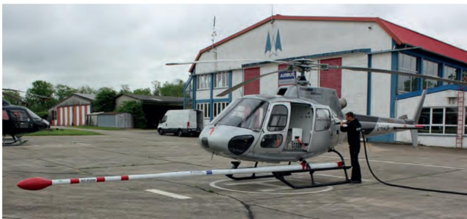
Image 5: Magnetics and radiometrics on AS 350 helicopter ready to take off.
