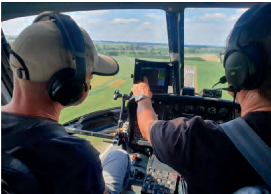
Image 4: Navigational display for flying accurate survey lines and altitudes.
